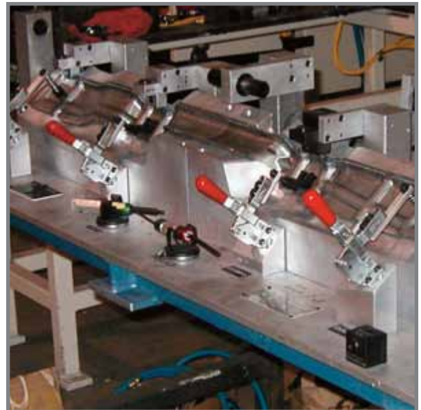
Model 210-U shown being used in a checking fixture application.
