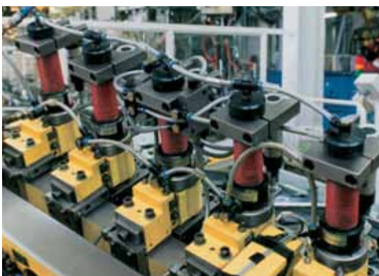
Stamping units placed in line
